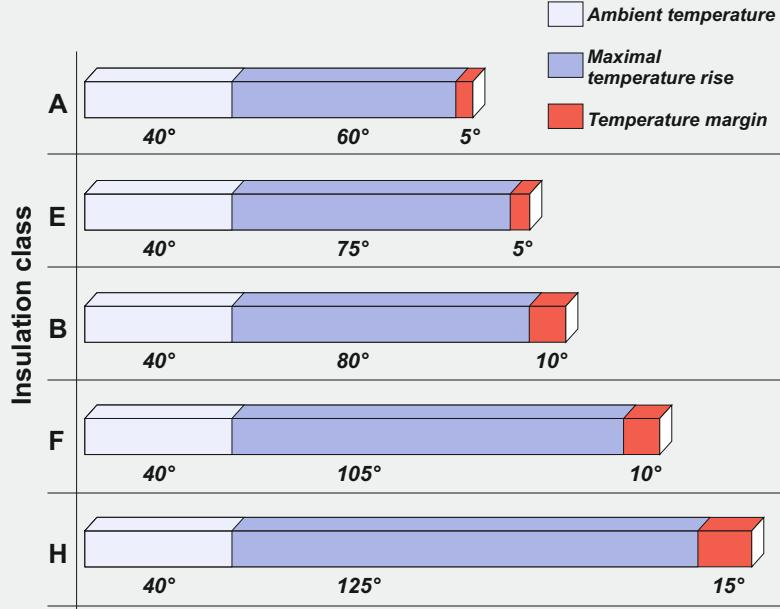
*Insulation class F in an electric motor means that at ambient temperature of 40°C the temperature rise of the winding may be max. 105°C with the additional temperature margin of 10°C (under specified measuring conditions in accordance with the IEC 60034-1 standard).*
